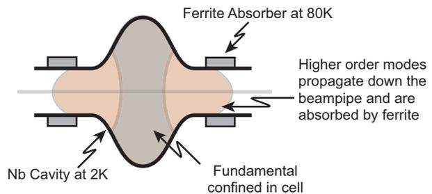
Figure 1: Schematic of Higher Order Mode absorber.
