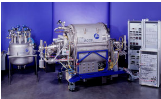
Figure 1: SRF accelerator module for the Taiwan Light Source with valve box (left) and SRF electronics (right).
