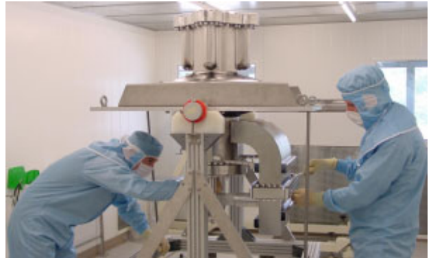
Figure 4: Preparation at ACCEL of a 500 MHz cavity for a vertical test. Up left: closed loop BCP, up right: high pressure rinsing, below: clean room assembly
