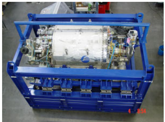
Figure 5: Completed 500 MHz module installed into shipping frame.
