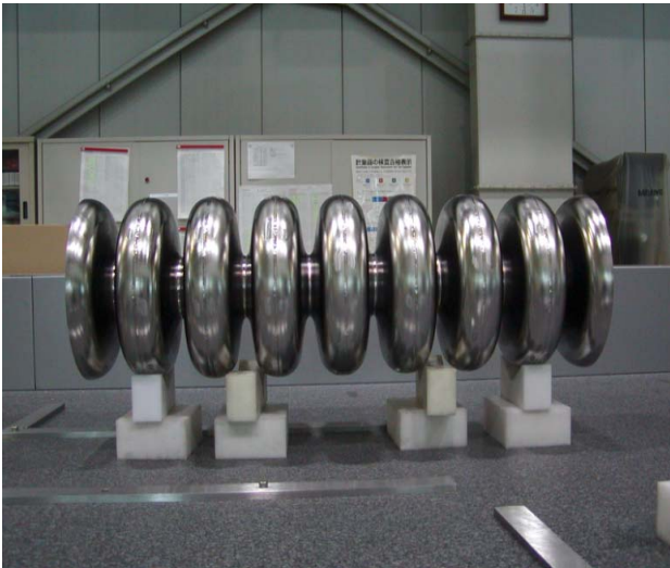
Figure 3: A welded center-cells.
