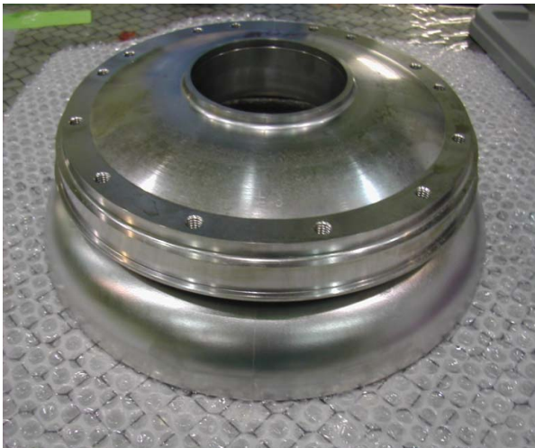
Figure 4: An end-cell with a titanium endplate.
