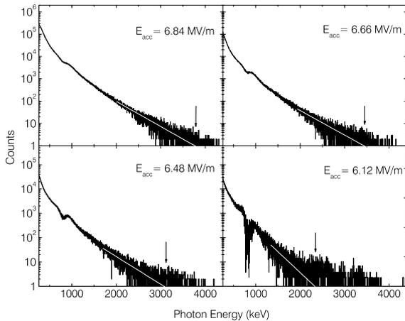
Figure 4: Bremsstrahlung spectra measured with a BGO detector for different accelerating gradients.
