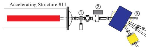
Figure 2: Experimental set up downstream of the main linac. The figures denote: (1) view screen, (2) BGO detector, (3) viewport for optical measurements.
