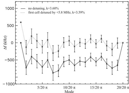
Figure 6: Difference between the measured passband frequencies and the calculated frequencies in case of a flat field profile (solid line) and in case of a perturbed field profile resulting from a detuned edge cell (dashed line).
