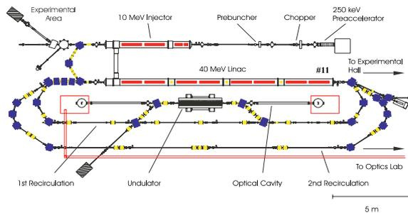
Figure 1: Layout of the S-DALINAC
