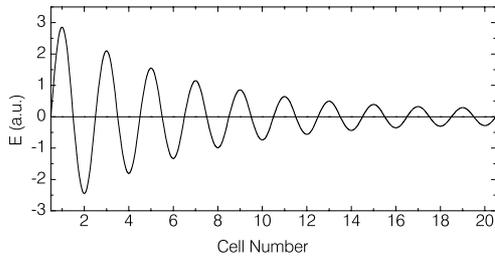
Figure 5: Field profile of a 20 cell S-DALINAC structure with the first cell detuned by 5 MHz.
